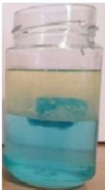
Figure 4. One must increase the density of the ice and add dish soap to the water to reduce surface tension. All these are necessary to come close to the theoretical result of the calculation of a usual physics exercise
