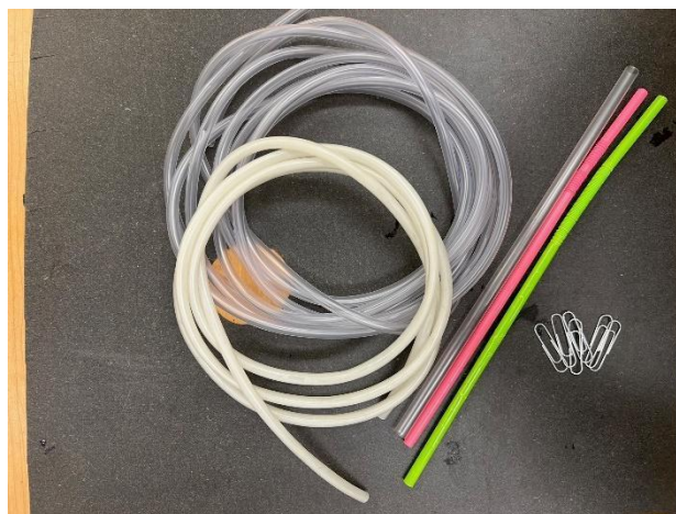
Figure 1. Materials needed for assembling the diver. Soft transparent tubes are a good alternative to plastic straws.
