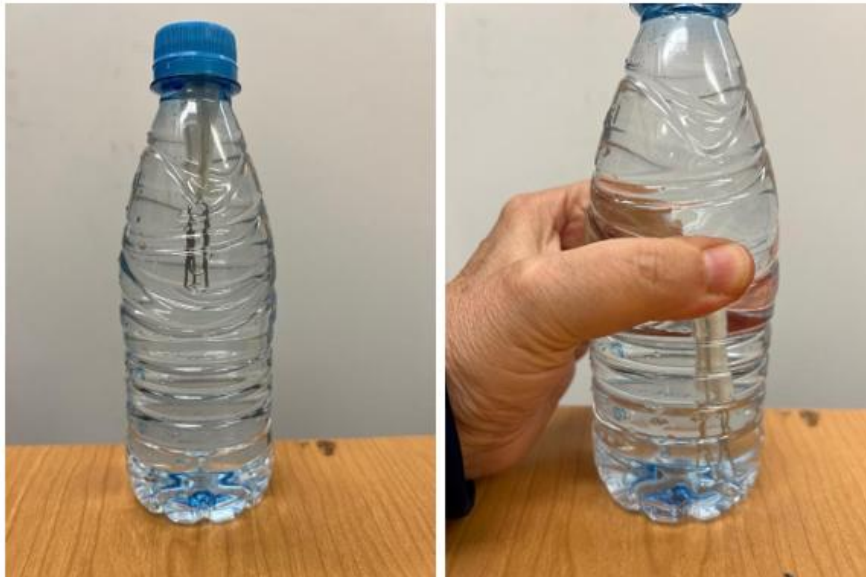
Figure 3. Left: Assembled Cartesian diver. The diver floats, if the PET bottle is not compressed. Right: Under pressure it sinks.
