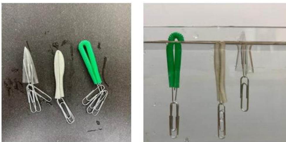
Figure 2. Left: Assembled Cartesian diver, the middle one is made from a rubber tube. Right: Floating Cartesian divers. It is evident that the diver from the rubber tube is heavier. This could be compensated by a longer part which contains air.
